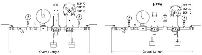
When using the Siemens SKP20 and SKP70 actuators for pressure regulating and ratio regulating functions, the sensing piping is not included. For proper operation, the sensing pipe should be at least 1/4" I.D. and connected a minimum of 5 pipe diameters downstream in a non-turbulent area. WARNING: For proper and safe operation, the installer must read and thoroughly understand the Siemens Technical Instructions 155-514P25 for the SKP20 and 155-516P25 for the SKP70.
